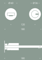
7305/3/A Miscelatore per lavabo a muro, L180 Wall mounted single lever mixer for basin, L 180
