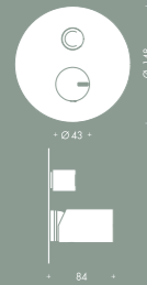
7300 Miscelatore incasso c/pulsante 2 OUT Built-in single lever mixer with diverter pulse 2 OUT
