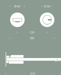
7305/3/B Miscelatore per lavabo a muro, L210 Wall mounted single lever mixer for basin, L 210
