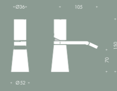
7307/S Miscelatore per bidet s/salterello Single lever mixer for bidet without pop-up waste
