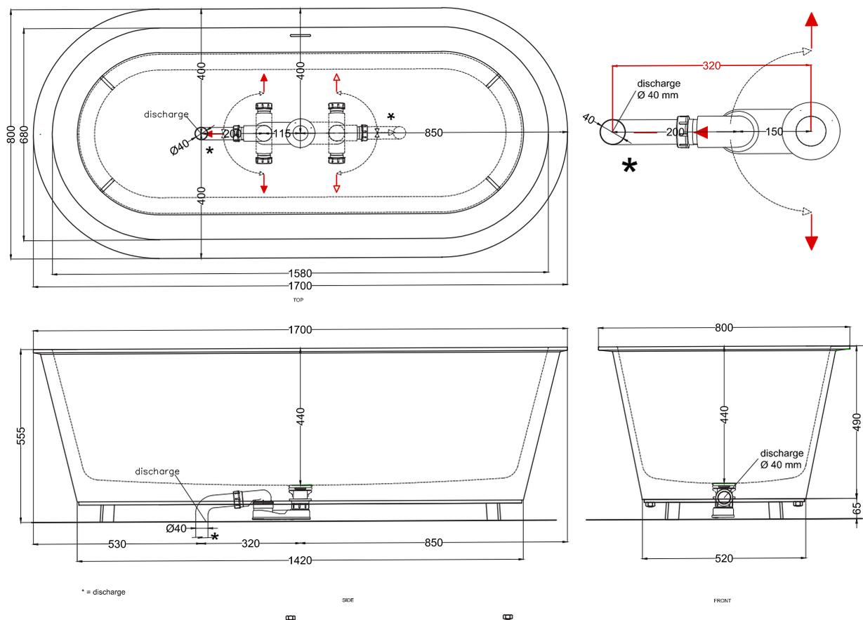
Allowed tolerance on dimensions after firing process:  $\pm 0.3$ mm
